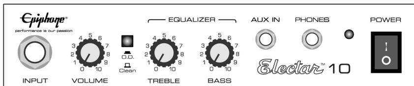
Your device is equipped with an external AC to DC power adaptor. First, plug the power adaptor's small cable end into the **Power IN** jack located on the back of the amplifier. Then plug the adaptor into your AC wall socket. Turn the power switch to ON. The RED LED should light up indicating power is supplied.
